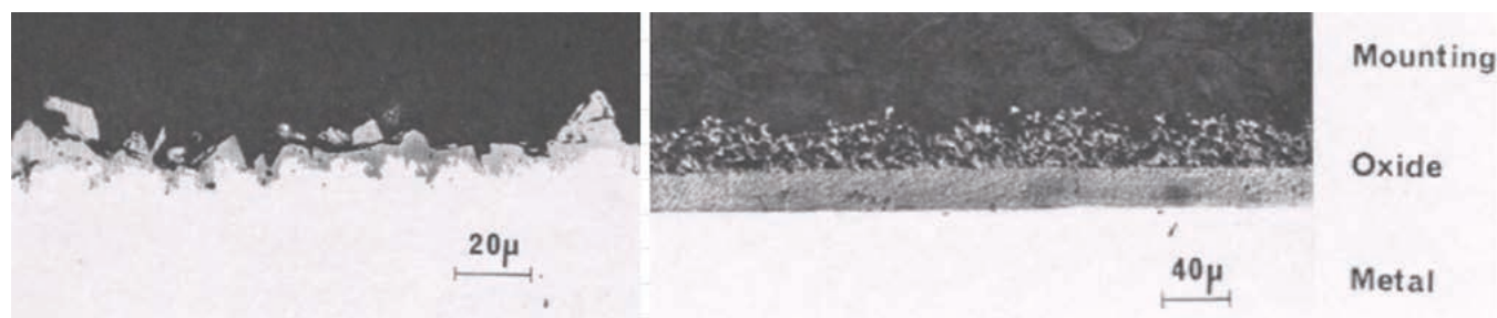
Figure 2: (Left) A very thin, 5- to 10-micron ( \mu\text{m} ), single-layered “Bloom film” made of large crystals fused to the surface. (Right) A very thick, 40- to 50- \mu\text{m} , double-layered “Potter-Mann film” with a compact underlying layer of small crystals and a loose top layer of large, well-formed crystals. (Figure 2 is from Reference 19.)
