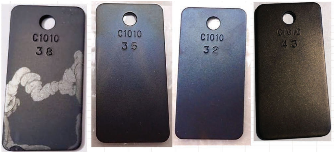
Figure 4: (Left to right) Unpolished mild steel coupons—untreated, TG3304, TG3124, and TG3106 treatments. The colors observed give an indication of the thickness of the films (40).
