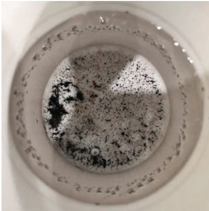
Figure 5: Detached magnetite at the bottom of the reaction vessel of the autoclave.
